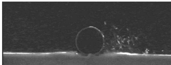
Fig. 5. Onset of sand scouring.
